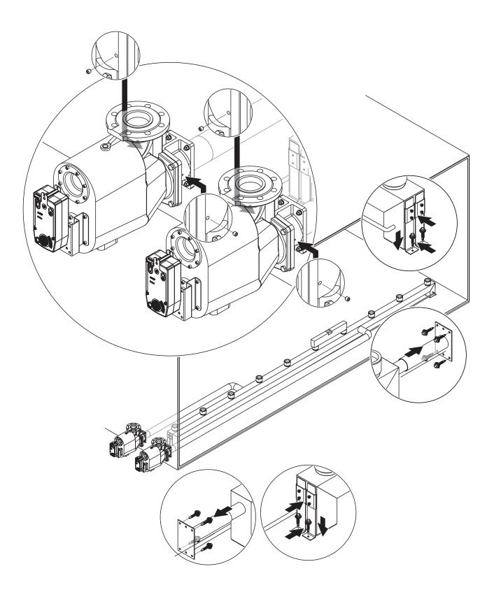
5. Seal the bores inside the duct with silicone-free sealant.
