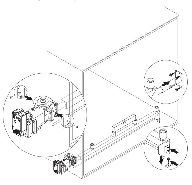
5. Seal the bores inside the duct with silicone-free sealant.
