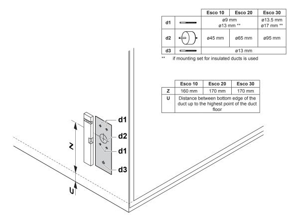
Use drilling template "1112848" for: Esco 10 with DR73 Use drilling template "1112849" for: Esco 20 with DR73 Use drilling template "1112850" for: Esco 30 with DR73
