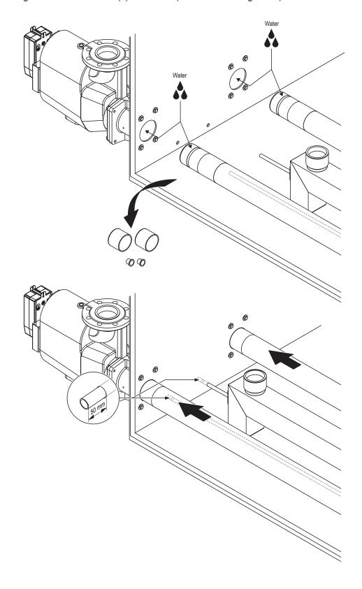
• If the valve unit(s) is(are) not mounted yet: from the inside of the duct push the connector(s) of the collector and the secondary condensate drain pipes through the corresponding bores in the duct wall until the connector(s) of the collector poke(s) **exactly T mm** out of the duct (see table below).
