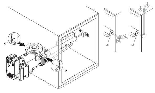
5. Seal the bores inside the duct with silicone-free sealant.
