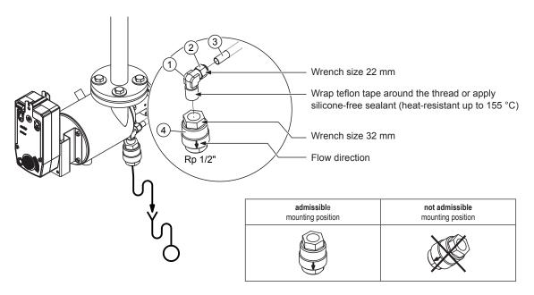
Push the threaded elbow connector (1) with the steam trap (4) onto the condensate pipe connector (3) and tighten the union nut (2) in accordance with the instructions below.
