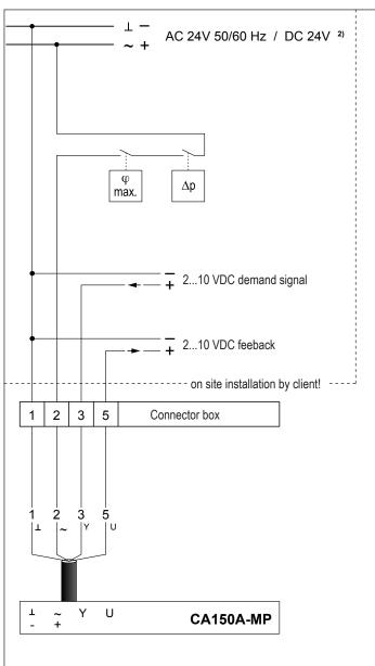
1) Caution! The two auxiliary switches in the actuator CA150A-S must be connected either to mains voltage or safety extra low voltage. The combination mains voltage/safety extra low voltage is not permitted!
