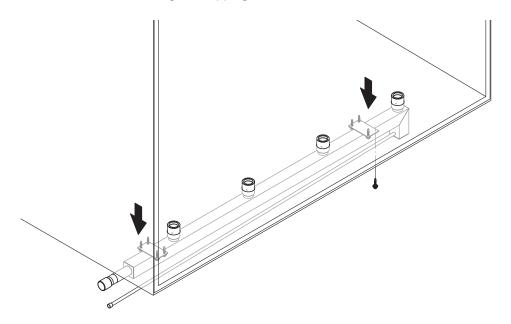
**Caution!** Until the definite supports are installed (step 4) the collector must be secured with auxiliary supports against falling down.
