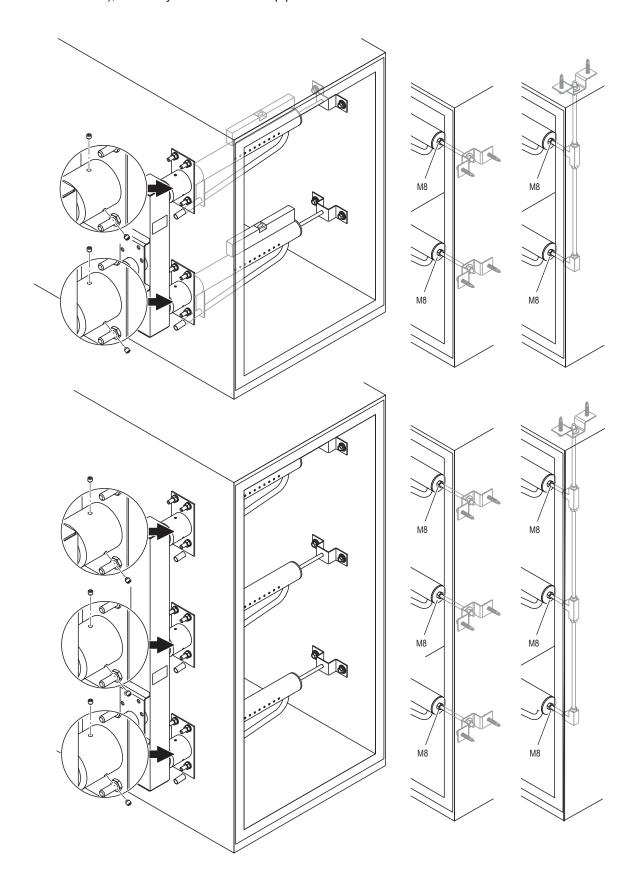
5. Seal the bores inside the duct with silicone-free sealant.
