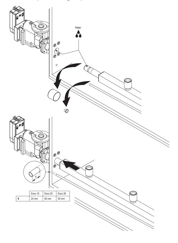
• If the valve unit is not mounted yet: from the inside of the duct push the collector and the secondary condensate drain pipe through the corresponding bores in the duct wall until the end of the collector pokes **exactly T mm** out of the duct (see table below).
