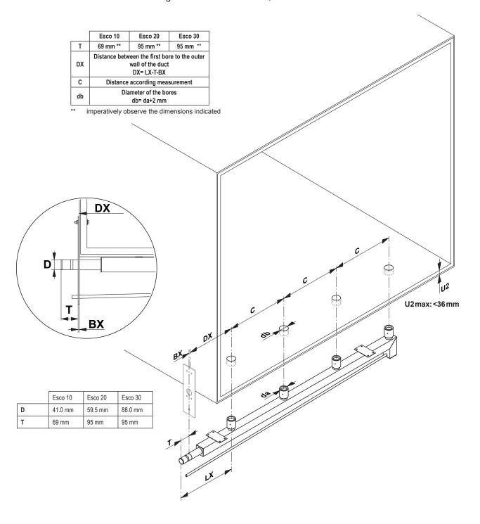
3. Fix collector to the duct floor using self-tapping screws.
