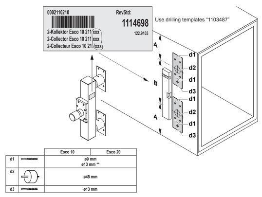
\*\* if mounting set for insulated ducts is used
