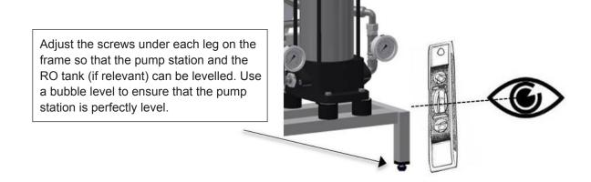
Fig. 12: Adjusting the pump station
