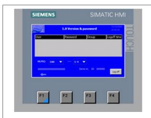
Select MLP size and select 1-4 or 1-8 sections. This selection is pre-set from factory according to the controller hardware.
