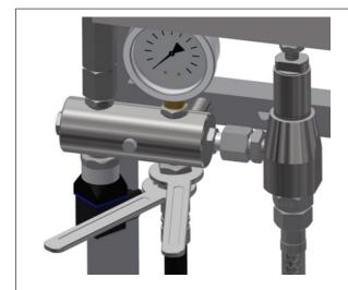
Turn S1 (on/off switch) to off position, and connect the HP discharge hose to the high-pressure manifold.
