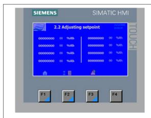
Force the HP pump to run by adjusting the set point in a section to 75%.
