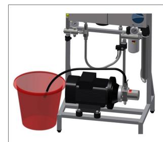
Remove plugs and strips from the highpressure hose and lead it to a drain or a bucket.
