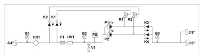
Fig. 8: Hydraulic diagram MLP 2x800
