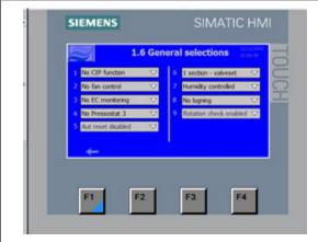
General selection between options and setups for the general pump station. Please note that some of the options require hardware that has to be ordered together with the pump.
