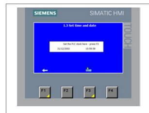
Time/date can be set (stored in the screen only). Note: Remember to press F3 to set the PLC clock
