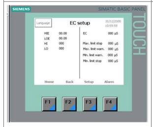
Setting the Alarm's and Warnings example, this sensor is choosen:
