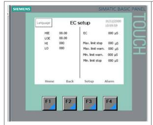
HIE, Input standard values, from chart, Overview of calibration for conductivity sensors and converters (amplifiers)
